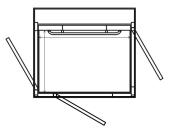
Configure your lift with doors on up to 3 sides over the whole travel of the lift.
