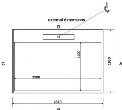
Hook in the building ceiling for 500kg, by builder, centred over guide frame. (Can be removed after installation.)
