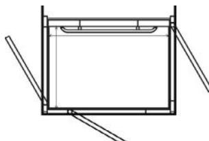
Configure your lift with doors on up to 3 sides over the whole travel of the lift.
