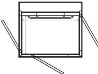
Configure your lift with doors on up to 3 sides over the whole travel of the lift.
